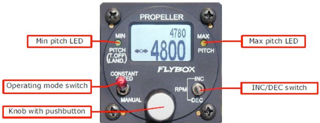
Fig. 7- 2: Constant Speed Controller Flybox
